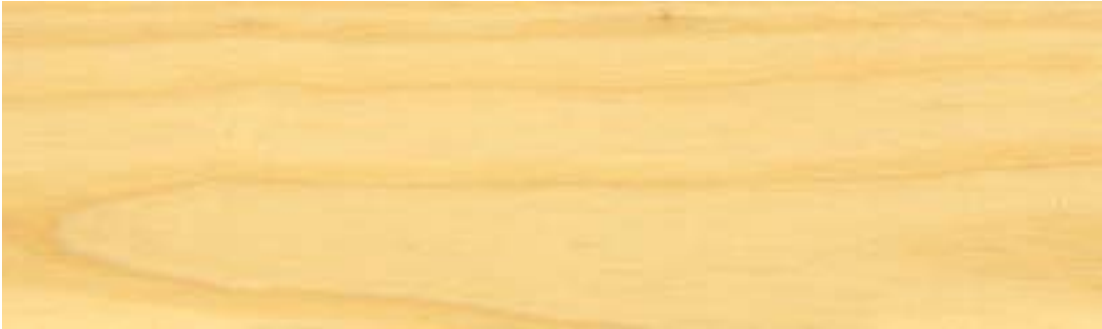
European White Ash Close-up of the Flat Sawn Graining
