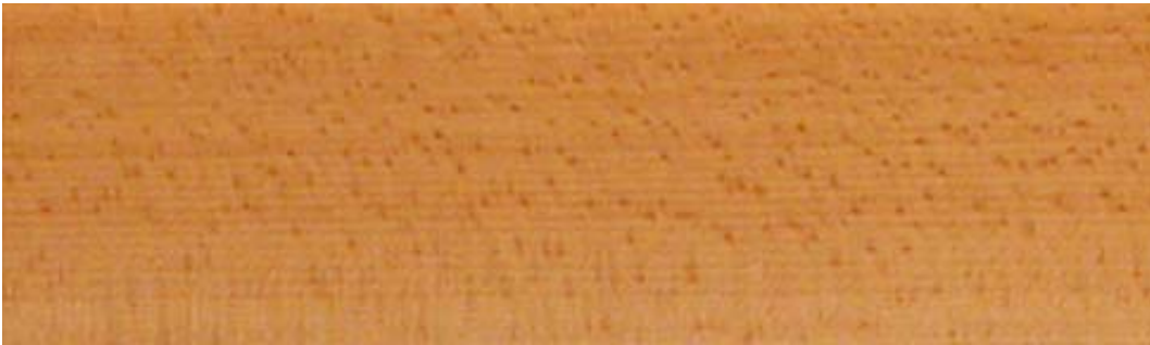
European Beech - Steamed Close-up of the Straight Grain / Quartered Graining
