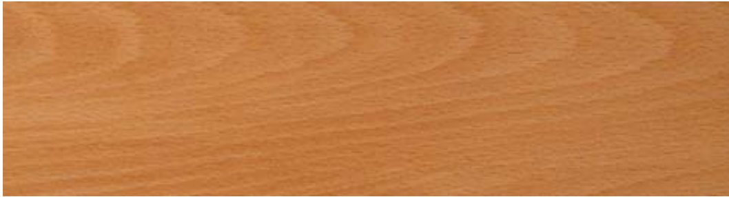
European Beech - Steamed Close-up of the Flat Sawn Graining
