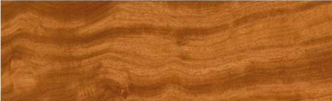
Doussie Close-up of the Flat Sawn Graining
