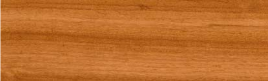
Doussie Close-up of the Straight Grain / Quartered Graining
